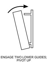
Figure 9. Attaching thermostat to subbase
